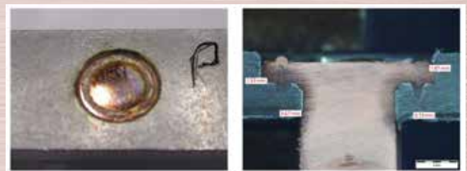
Figure 5) Electrical contact welding sample. Left: as-welded condition. Right: Cross section of welding for comparison with OCT-results.
